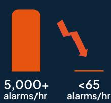
Chattering issues were handled with delay timers, deadband duplicates were eliminated through rerationalization, and suppression groups were developed for both planned and unplanned events to prevent alarm flooding during critical operations.
