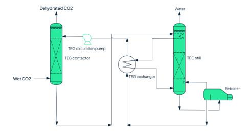
Triethylene glycol (TEG) dehydration is a widely used method for removing water vapor from natural gas and other gas streams, including CO2 in carbon capture processes. This technique prevents the formation of hydrates and reduces corrosion in gas transportation and storage systems.
